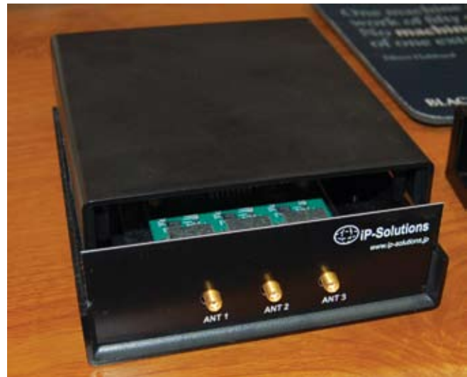
FIGURE 15 Special RF recorder with two synchronized recording tracks for high-sensitivity and multipath research
